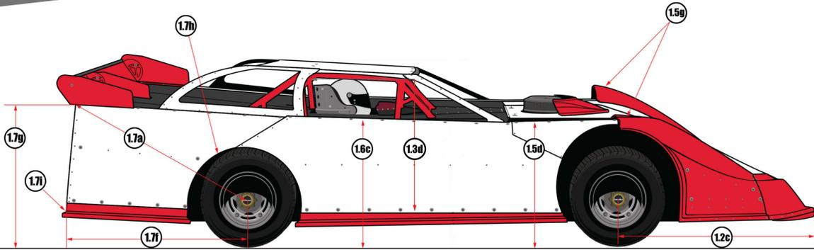
**1.2c** Stock nosepiece can extend a maximum of fifty-three inches (53") from center of front hub to farthest point extending forward
