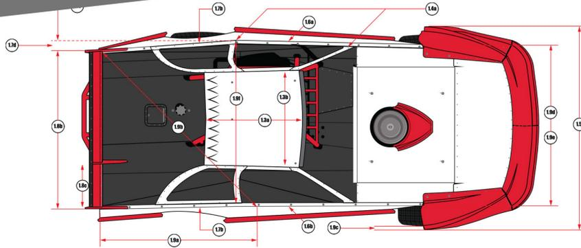
**1.3a** Roof length must be a minimum of forty-four inches (44") to a maximum of fifty-four inches (54")
